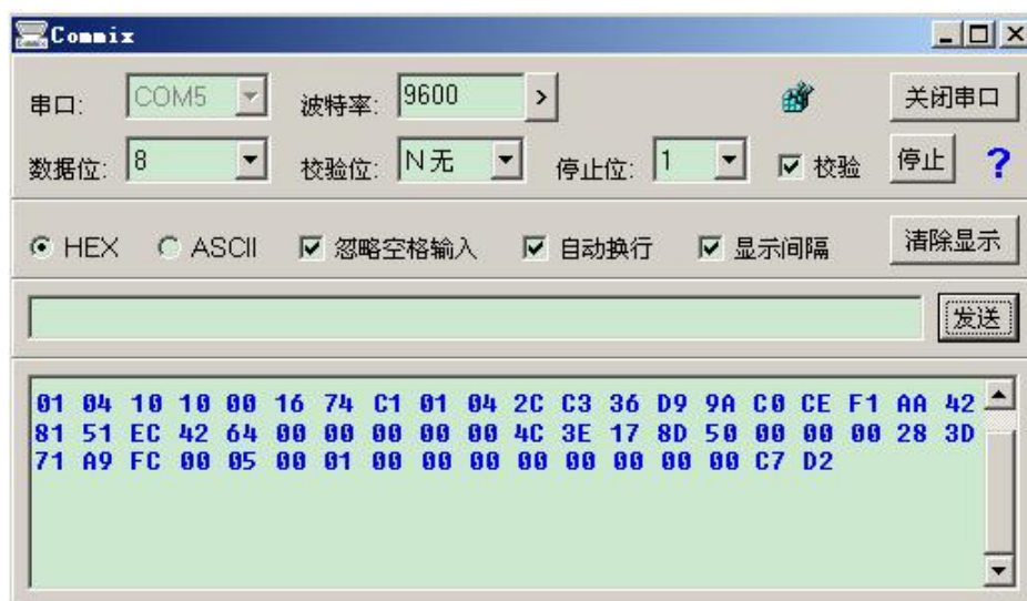
Figure 6-4 Example of Serial Port Debugging Assistant Listening
