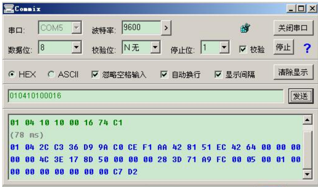
Figure 5-1 Communication Diagram of Serial Port Debugging Assistant
