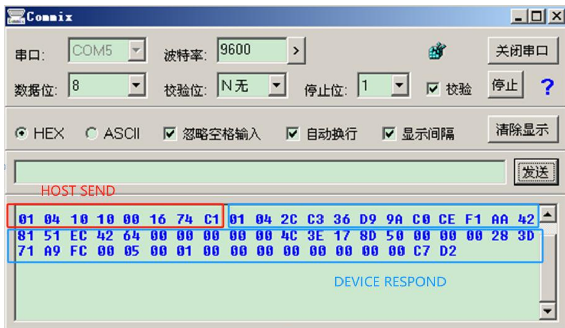
Figure 6-5 Example of Data Analysis for Serial Port Debugging Assistant
