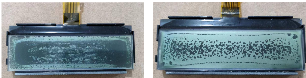
FigF10.1 After a long time of direct sunlight, the LCD module cannot display normally
